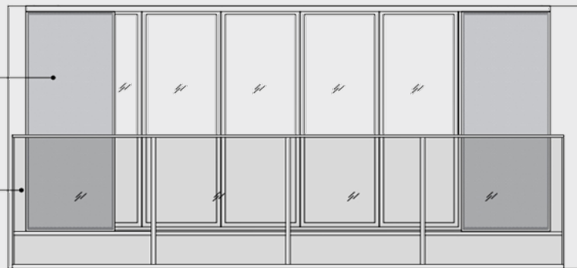
ELEVATION 1 (BALCONY SCREEN OPENED POSITION)
